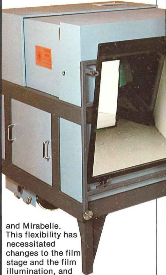
and Mirabelle. This flexibility has necessitated changes to the film stage and the film illumination, and a complete re-design of the operator console.
