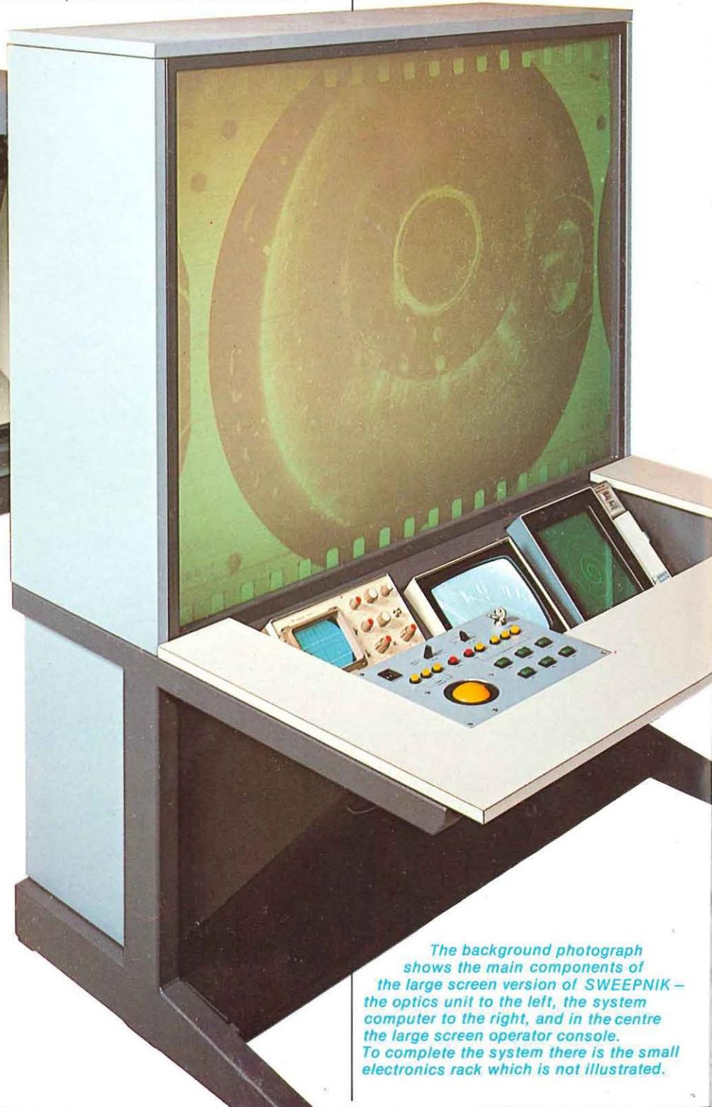
*The background photograph shows the main components of the large screen version of SWEEPNIK – the optics unit to the left, the system computer to the right, and in the centre the large screen operator console. To complete the system there is the small electronics rack which is not illustrated.*
