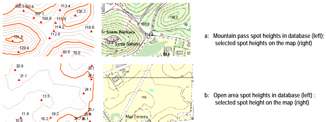
Figure 8: Spot height selection in terrain context - (thanks to ICC for the data and specifications)
